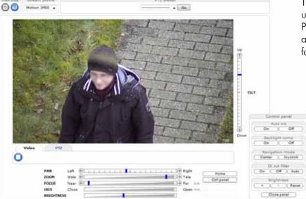
The person was detected by the radar unit. The coordinates were sent to the PTZ camera and the focus was adjusted to the person's torso and face. Identification becomes possible.
